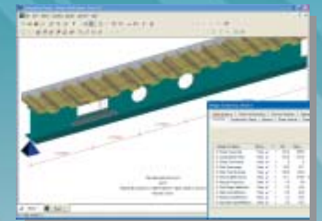
▶ Complete design including stiffened web openings
